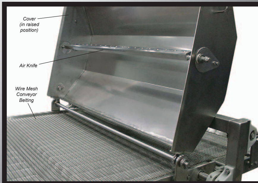
Transfer Conveyor With Cover Open
