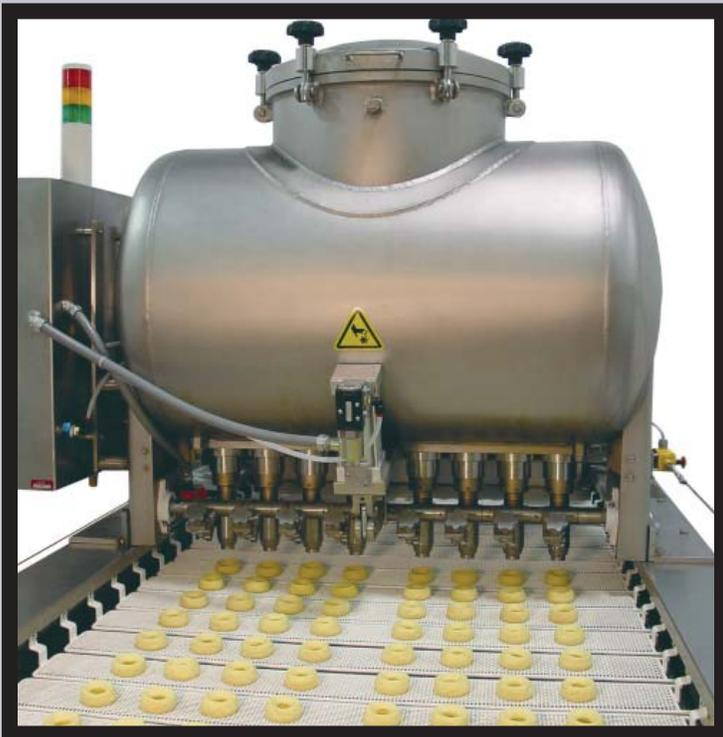
Cutters Mounted on a Moline Yeast Raised Pressure Depositor
