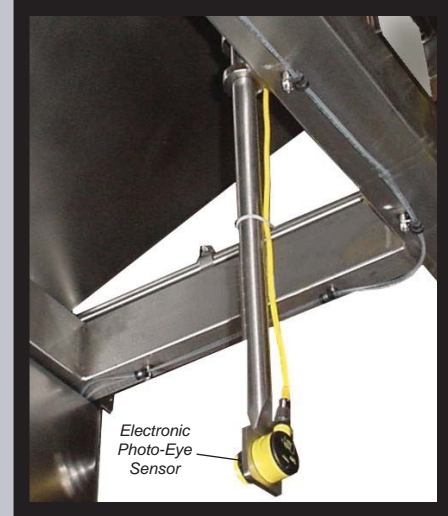
Dough Sensors on Chunker Frame
