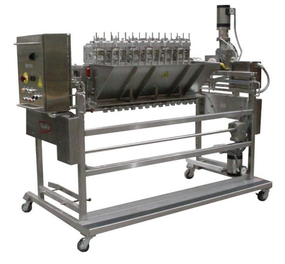
The Moline DonutKing Depositor is designed to continuously and uniformly cut and drop cake donut batter into a fryer kettle. The depositor consists of the following assemblies and systems: the hopper, the cutter head (and plunger) drive system, the bridge lifting system, the pneumatic system, and the electrical control system. Product size is easy to regulate by turning the cutter head adjustment knob.
