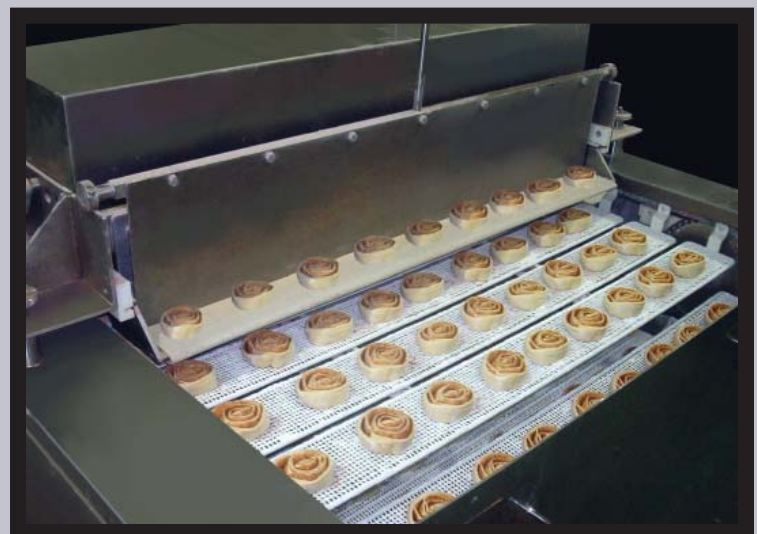
Shuttle Delivering Product to Proofer Trays
