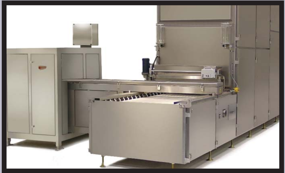
Transpositor Installed at Proofer Infeed Section
